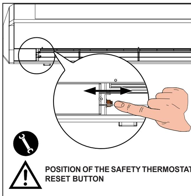
In the event the manual rearm protective device intervenes, the system will need to be restored only after having cut power and found out the cause of the fault (intervention reserved for maintenance operators alone).
