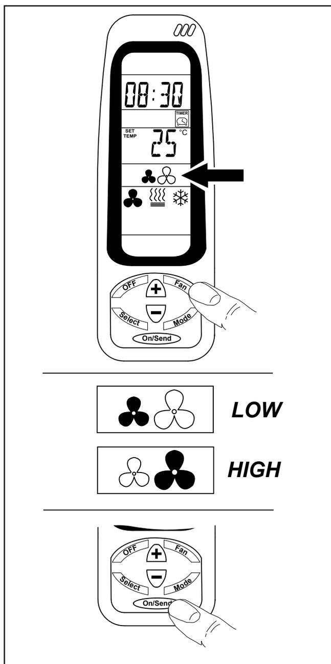
Press the **FAN** button to select the desired fan operating speed:
