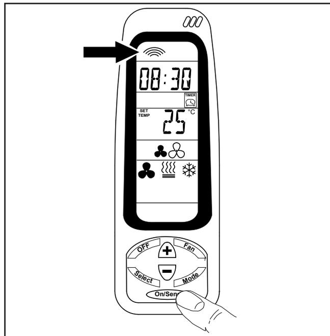
Whenever the operating parameter need to be modified, the instructions must be sent to the unit by pressing the “ON/SEND” button.
