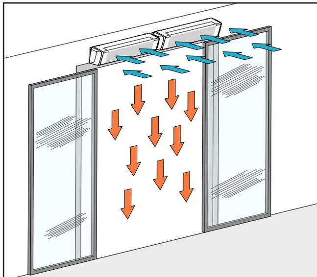
The efficiency of the air curtain depends on the air temperature, pressure differences across the doorway and any wind pressure.
