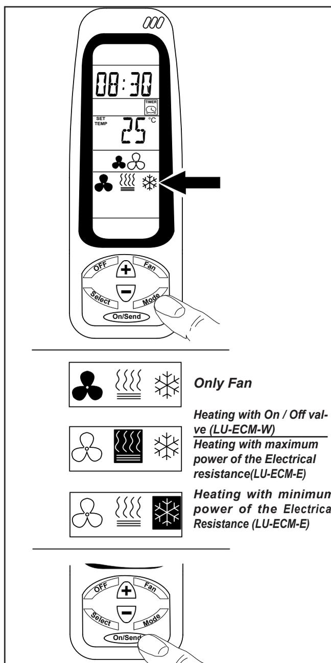
Press the **Mode** button to select the desired operating mode: **FAN or HEATING**.
