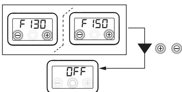
Press the "+" switch and the "-" switch in the same time in oder to activate the unit again.
