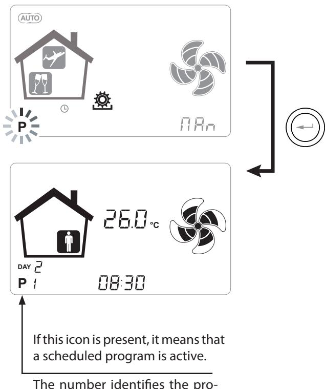
The activation of the weekly program does not preclude the user's ability to manually change the speed of the fans.
