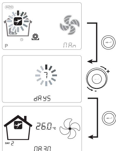
In Holiday mode, the unit operates at the minimum ventilation flow rate.
