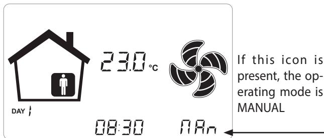
With the "Manual ventilation" mode enabled, the speed of the fan at the various points can be adjusted by scrolling with the **TOUCH PAD**. Turning the key clockwise on the pad increases fan speed, while anticlockwise decreases fan speed.
