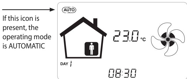
When the "**Automatic Mode**" is enabled, fan speed is controlled by an automatic control cycle relative to internal instantaneous variations of the measured air quality variable (default humidity). See specific section for more information
