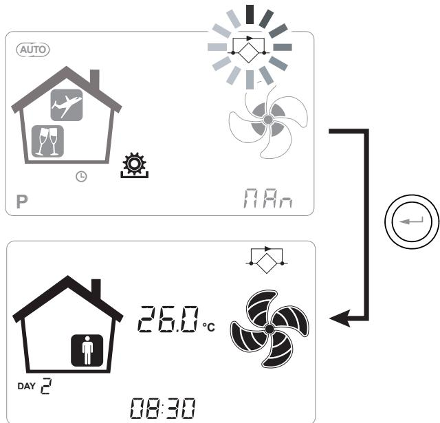
**ATTENTION!**: In order to end FREE-COOLING and restore heat recovery, change the mode manually by accessing the user screen.
