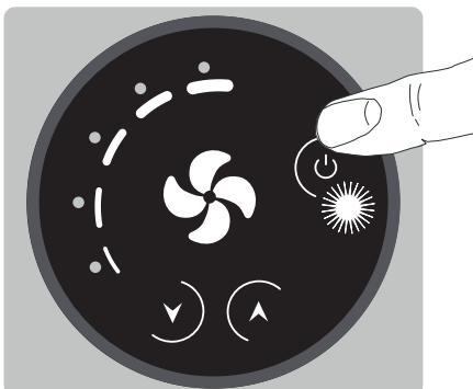
The button allows to activate the device or put it in stand-by mode.
