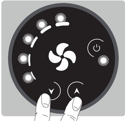
*During stand-by the brightness of the LEDs will be halved compared to the chosen value.*
